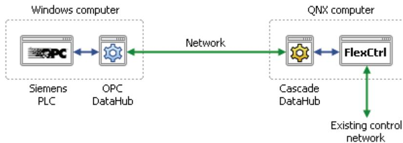
The Servers and communication-servers and a part of the control-stations are running QNX. The other part of the control-stations is running Windows. The control there is via Phindows (graphical terminal). The data are also exported in different formats for further processing in other systems.
