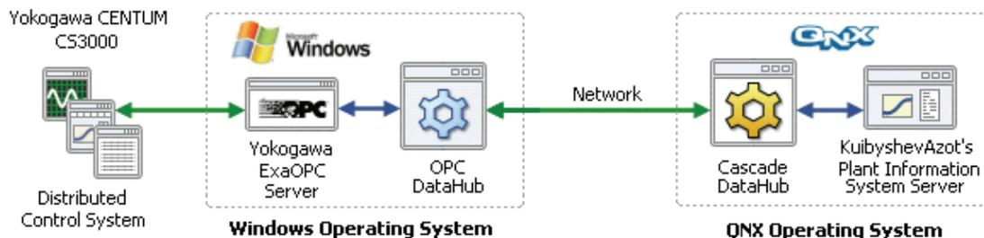
Each of these DataHubs is an off-the-shelf middleware program that collects and distributes real-time data. The OPC DataHub runs in Windows, and can connect to any OPC server, such as the Yokogawa ExaOPC Server used in the project. On the QNX side, the Cascade DataHub was connected to the Plant Information System server. Once connected to their respective systems, the two DataHubs establish a TCP mirroring connection across the network to create a Windows – QNX real-time data link.
