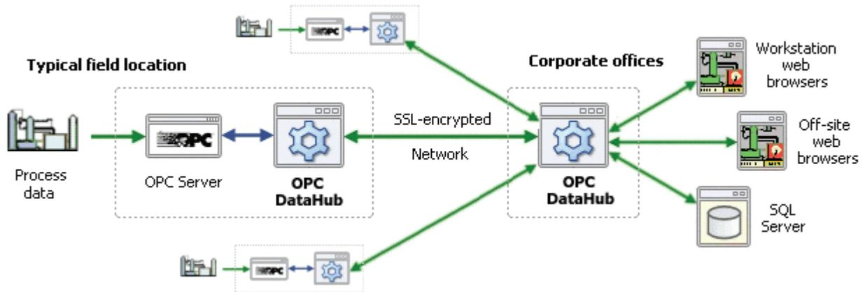
Using Java applets that come with the OPC DataHub, Robert created a web page that displays live data overlaid on top of a system diagram, along with a table showing status messages and alarms. Then he configured the DataHub to write data to his SQL Server database. Finally, he installed an OPC DataHub in the central office, and configured a secure, SSL-encrypted tunnel between the two DataHubs to mirror the data.
