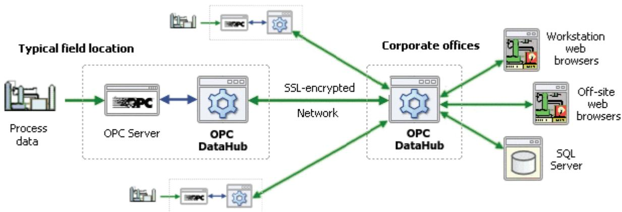
Using Java applets that come with the OPC DataHub, Robert created a web page that displays live data overlaid on top of a system diagram, along with a table showing status messages and alarms. Then he configured the DataHub to write data to his SQL Server database. Finally, he installed an OPC DataHub in the central office, and configured a secure, SSL-encrypted tunnel between the two DataHubs to mirror the data.
