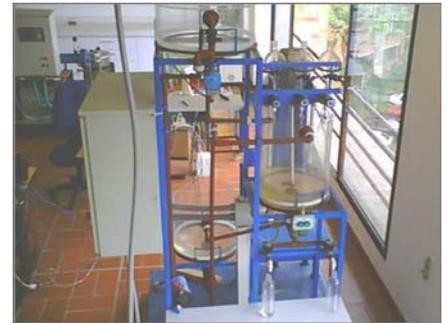
Recently, graduate students Andres Mora and Juan Guillermo Botero have been using Rockwell's FactoryTalk View SE Studio to design a SCADA system for the project. The three simulated plants are connected by ethernet to a single Unitronics OPC server, and the plan was to then connect that to the SCADA system's OPC client.
