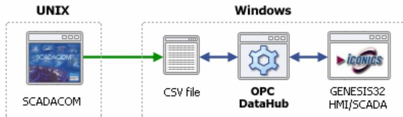
Starting with a demo script from the OPC DataHub archive, Mr. Munoz has been able to access data from a legacy UNIX system and make it available through OPC. To access the data, Mr. Munoz wrote a DataHub script to read a CSV file every minute and write the values to points in the OPC DataHub. Because the OPC DataHub is also an OPC server, this allows points from the UNIX system to be presented as OPC tags to the HMI system.
