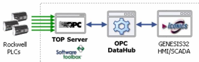
“The OPC DataHub effectively decouples the OPC server from the client,” said Mr. Munoz. “All the load is on the DataHub's shoulders now, and the performance is much better.” The TOP Server is now free to optimize the communications to the device while the OPC Data Hub protects it from device reads. This has relieved the company from having to redesign their HMI and PLC configurations from the ground up, saving them tens of thousands of dollars in engineering and development work.
