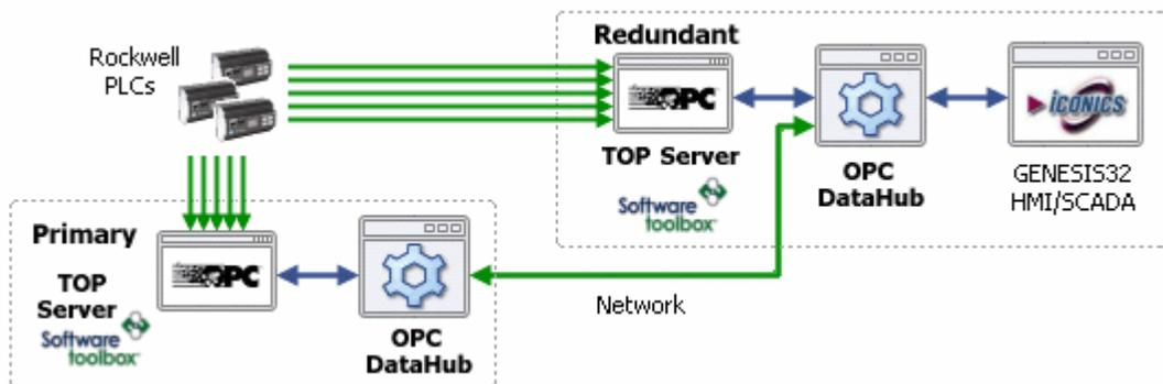
The most recent project that Mr. Munoz has decided to tackle with the OPC DataHub is to implement redundancy. To provide increased availability, the company has installed an additional OPC server at some locations. Working with Win Worrall, Product Support
