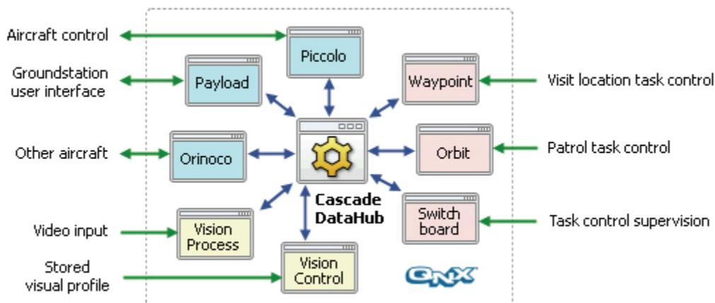
For example, the communication software comprises three separate processes: The piccolo process controls the aircraft, the payload process communicates with users on the ground, and the Orinoco process handles communications with the other aircraft. Needless to say, each of these three programs needs information from the other two, as
