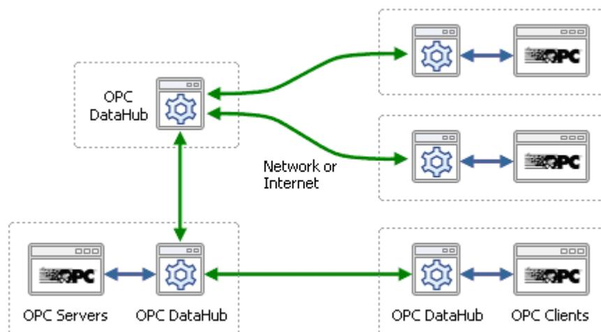
Load Balancing using the OPC DataHub
