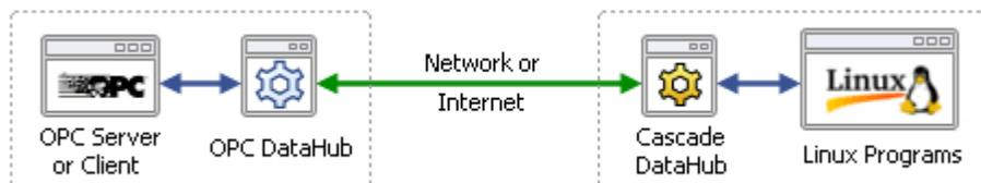
Connecting OPC to Linux using the OPC DataHub
