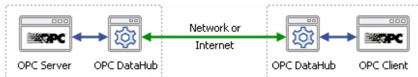
Tunnelling data using the OPC DataHub
